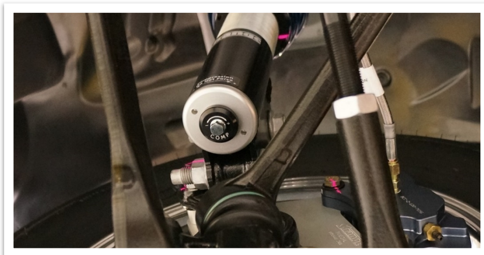
Front Compression Adjustment (Clockwise = More Damping)
